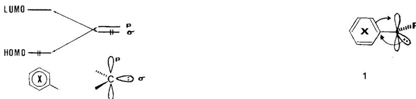
Fig. 1. Schematic representations of the interactions between arene MO's and a carbene substituent
